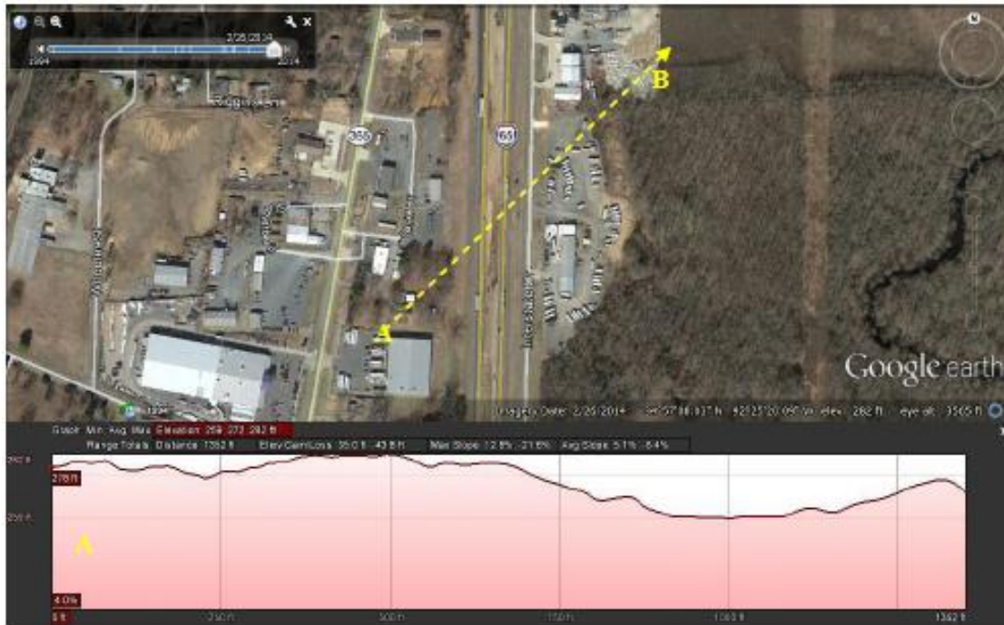
Fig. 26 Elevation profile for line AB at interstate I40 where it is hit by the tornado.
