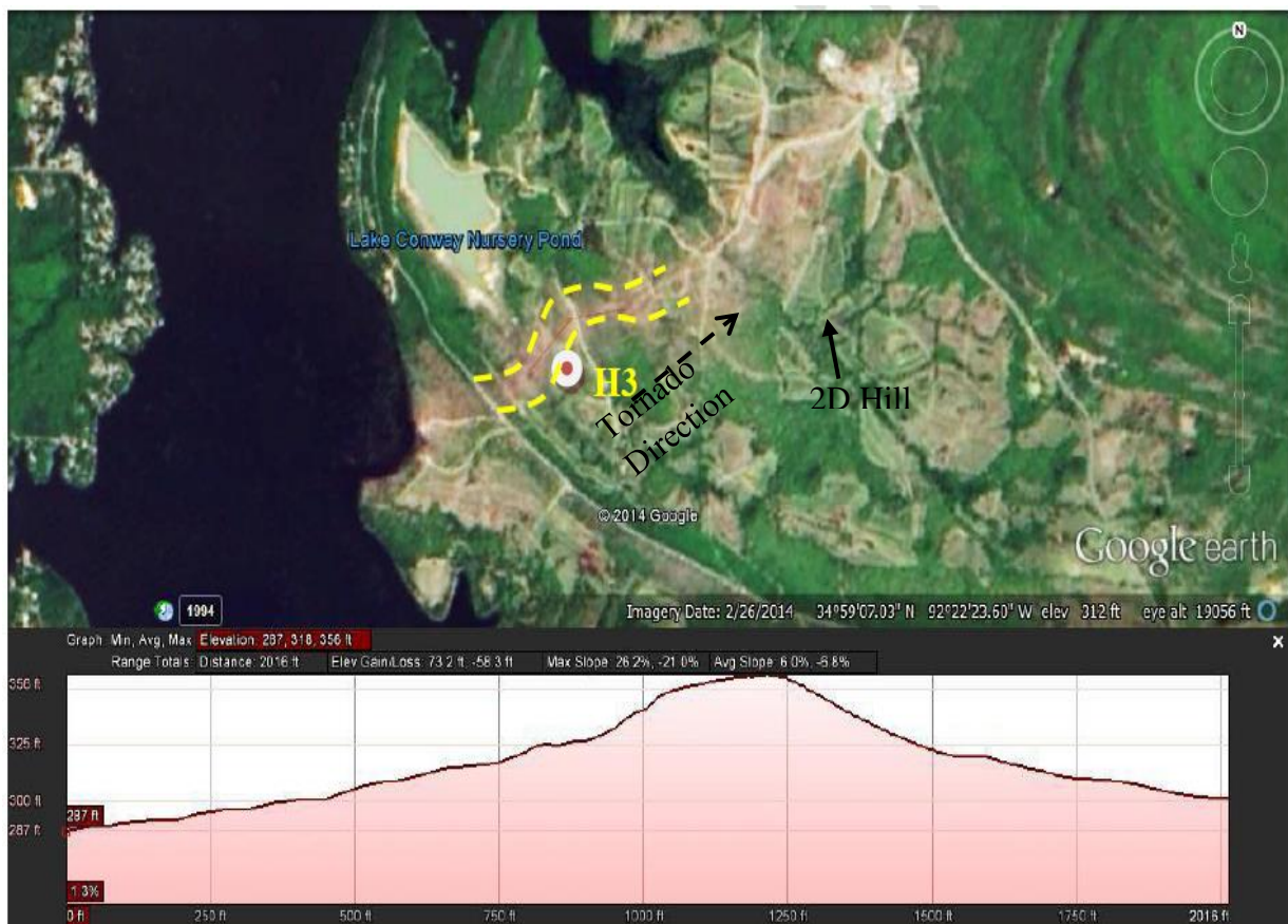
Fig. 10 Elevation profile for the hill in location H3, ( V_0/V_t \approx 4 , single curvature).
